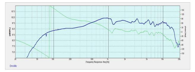
The notch in the woofer's response at 1200 Hz is real. It is most likely due to the cone's edge resonance where it terminates to the soft rubber surround. In my opinion though it is not an issue to be concerned with, as narrow band notches are generally inaudible, and I have never noticed anything in my listening sessions that I would attribute as an issue in this frequency range.
