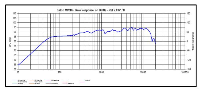
I measure the exceptional bandwidth of the driver too; the only other real difference between my measurement and the SBA graph is that my measurement shows the baffle step and hump associated with the driver being measured on my 9" x 16" baffle. This chart shows  $1/48^{th}$  octave smoothing.
