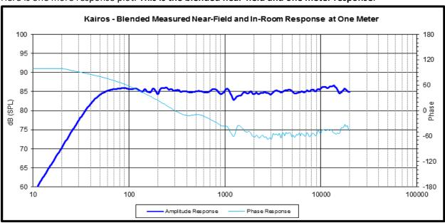
Here is one more response plot. This is the blended near-field and one meter response.
