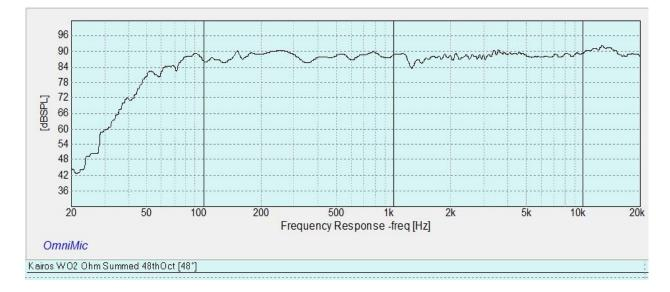
**Here's a plot of the actual measured acoustic crossover**. As you can see, it matches the plot above perfectly. The data in this graph is good to about 300-400Hz, below that the room begins to take over. This can be seen in the graph, but its purpose is intended to show the actual measured acoustic crossover response and summation of the drivers:
