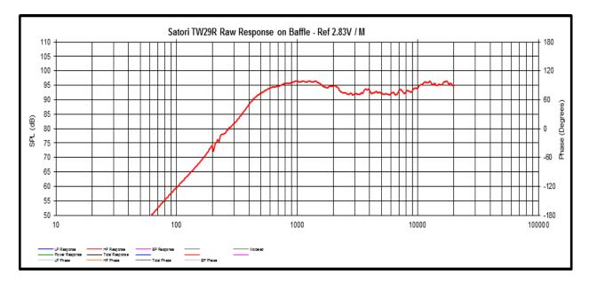
The broad hump centered at 1 kHz is due to baffle diffraction, but this is very easy to accommodate in the crossover design. As you can see, this tweeter has strong output down to 500 Hz, and relatively high sensitivity.
