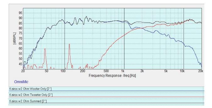
**For those that are interested, here are the actual filter transfer functions.** The early initial roll-off of the woofer's filter is for the purpose of compensating for the baffle diffraction step. The measured response shows how well this simple curve flattens the response:
