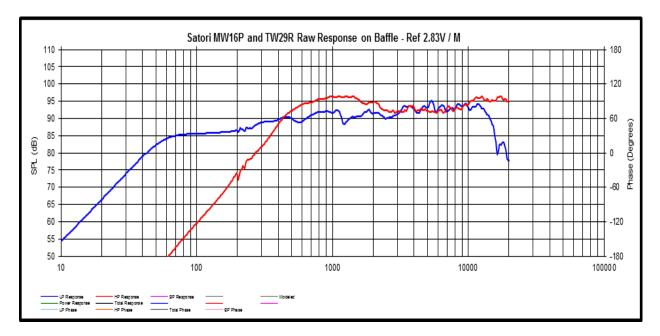
The graph above shows the raw frequency response of both the woofer and tweeter measured under identical conditions on a 9" x 16" baffle. This demonstrates the broad overlap in their frequency response. Based on this overlap and the linear, low distortion behavior of the drivers I opted to design a speaker that is time and phase accurate as well as one that has flat extended frequency response.
