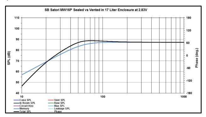
Here is a graph showing the difference in the response between the vented and sealed modes of the speaker.
