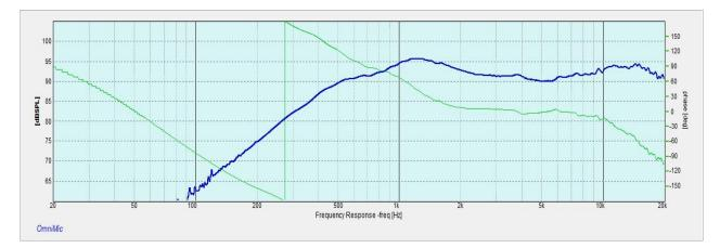
Part of the hump at 1200Hz is due to baffle diffraction in my set-up, so you need to ignore some of that, and even though my scale is compressed a bit from SB's, the two curves match up very well .
